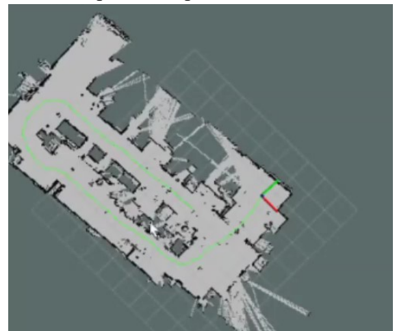
Figure 9: Sample 2D map from LIDAR data. The green line represents the estimated MAV trajectory.
